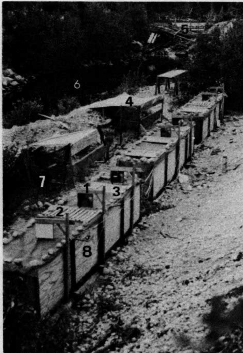
Fig. 1 - General view of the experimental installations. 1- Food distributors. 2- Screen over semi-shaded area. 3- Opaque screen. 4- Observer hideout. 5- Dam and resulting pond. 6- Castor Noir brook. 7- Camouflage net. 8- Artificial stream.
