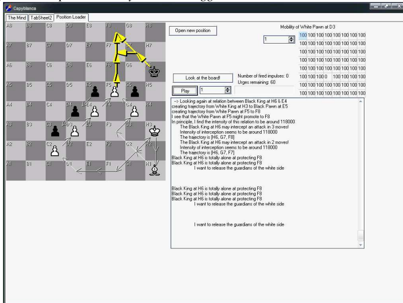
Figure 10. After codelet 396, all white pieces' 'guardian' roles have very low intensity. For example, intensity of white bishop's defense of the g4 pawn is less than 1/10000 of the intensity of the potential pawn promotion—the reader should note that an arrow's thickness display is affected by orders of magnitude.
