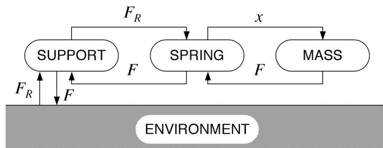
Figure 3.4: Oscillator UC-structure.
