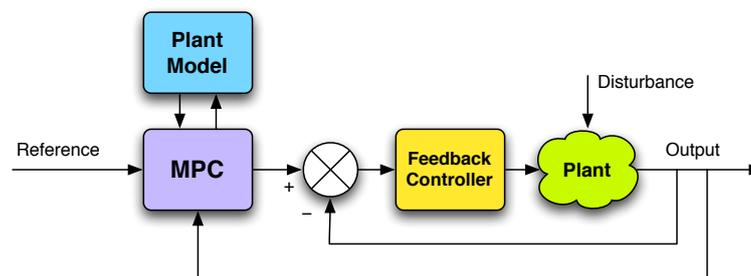
Figure 1.2: Schema of a model-predictive control
