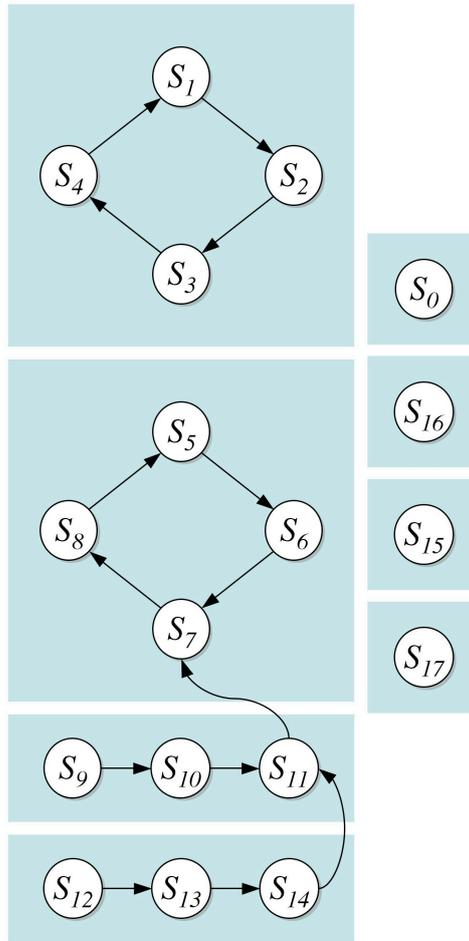
Figure 3.9: Oscillator ST-structure.
