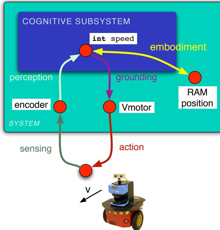
Figure 3.14: Example of grounding and embodiment concepts in a mobile robotics application
