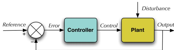
Figure 4.2: Feedback controllers measure the difference (error) between what we want (reference) and what we have (output) and make corrections (control) based on this difference.
