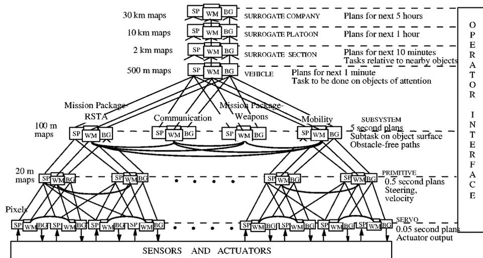
Figure 6.1: Example of a RCS hierarchy from [Albus et al., 2002], in which there can be appreciated the different resolution levels
