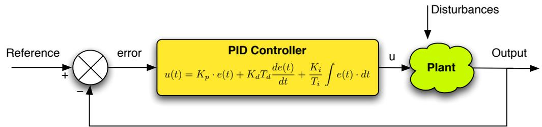
Figure 1.1: The PID controller
