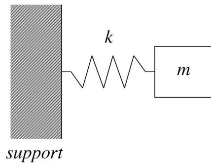
Figure 3.3: Mechanical Oscillator. A mass  $m$ , coupled to a spring of rigidity constant  $k$ , coupled to a fixed support.
