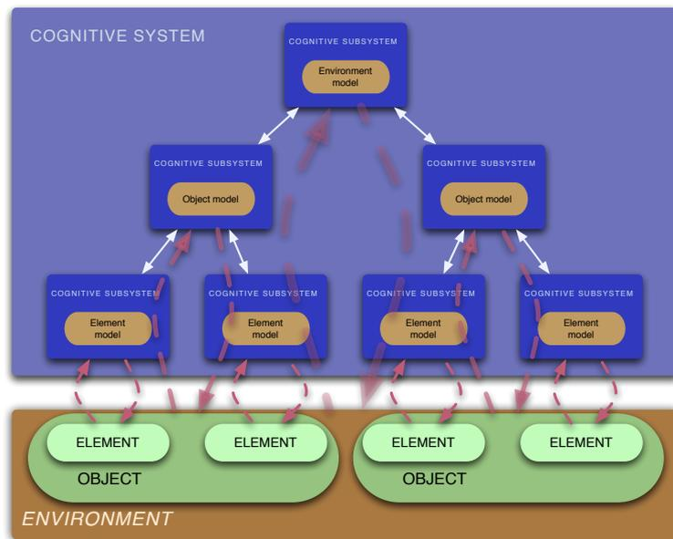
Figure 4.3: Complex cognitive systems in integrated control architectures need to exploit models in the performance of tasks at different levels of abstraction; from the immediate reaction to environment changes to the strategic decision making relevant for the long term performance of the system.
