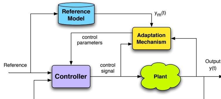
Figure 1.3: Architecture of a MRAC controller
