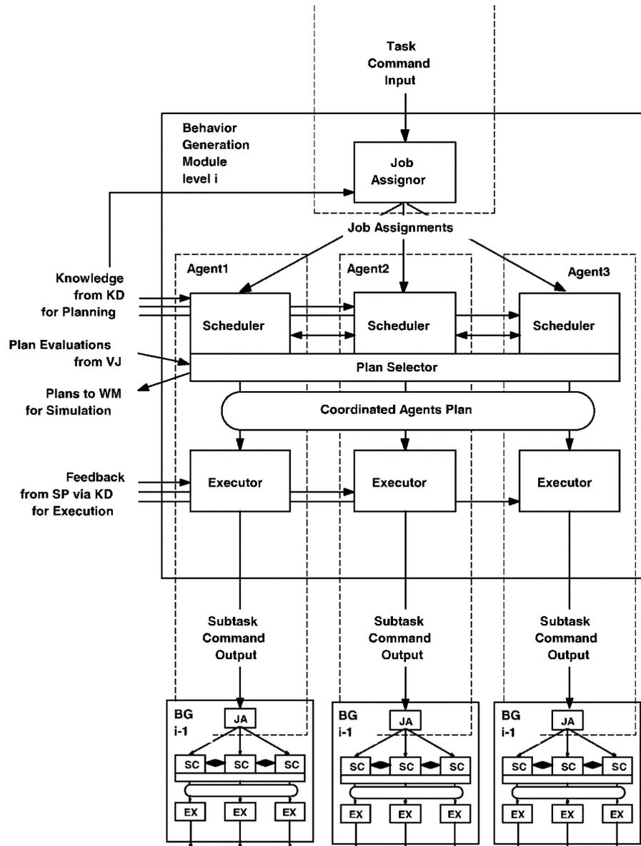
Figure 6.4: Internal structure of Behaviour Generation [Albus et al., 2002]
