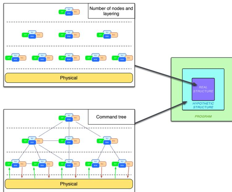
Figure 6.5: RCS layering and command tree
