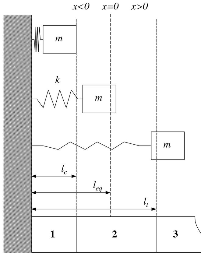
Figure 3.5: Regions of Operation of Oscillator.  $l_c$ – length at maximum compression, when the spires of the spring are adjacent to each other.  $l_{eq}$ – length at the equilibrium point of the spring,  $x = 0$ .  $l_t$ – length at the limit of elasticity of the spring.
