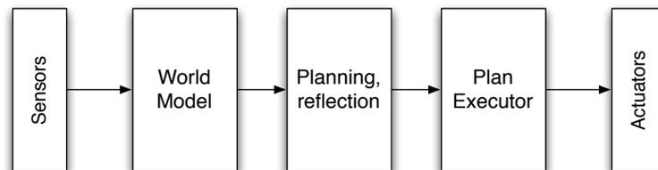
Figure 2.1: The common structure of a deliberative architecture.
