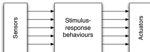
Figure 2.2: The reactive architecture
