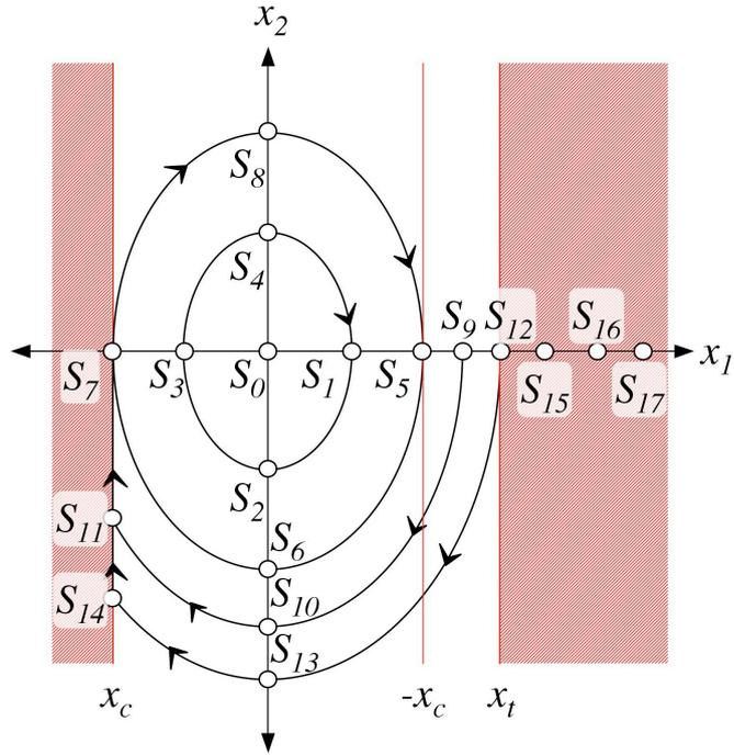
Figure 3.8: Oscillator Typical States.
