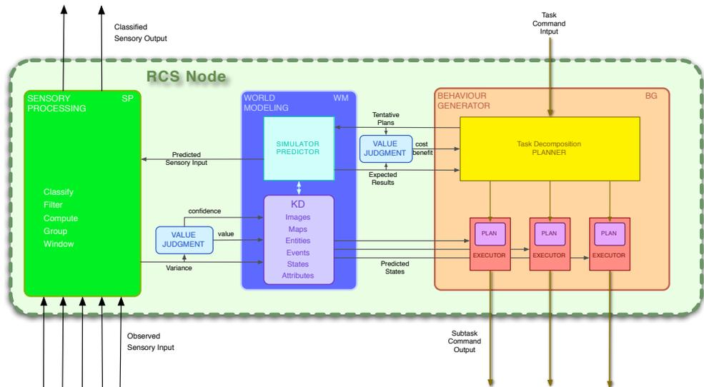
Figure 6.2: Functional structure of a RCS node
