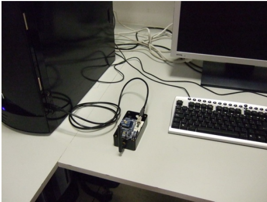
Fig. 15 Coordinator connected to a Computer USB Port in Lab 1.2
