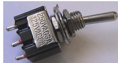
Figure (14): Three terminal on-off switch
