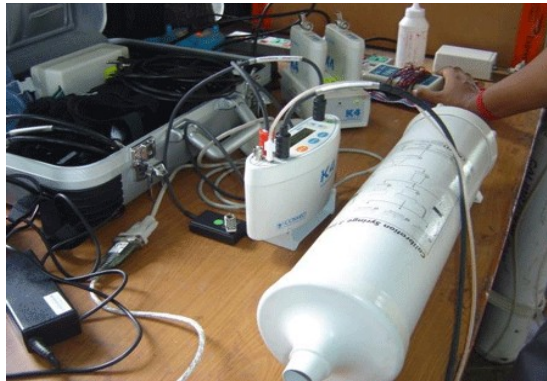
Figure 1: Cosmed® K4 B2 Respiratory Analyzer system
