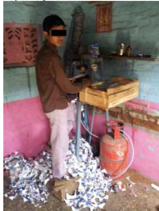
Figure 1: A Padia worker working on a Padia making press.
