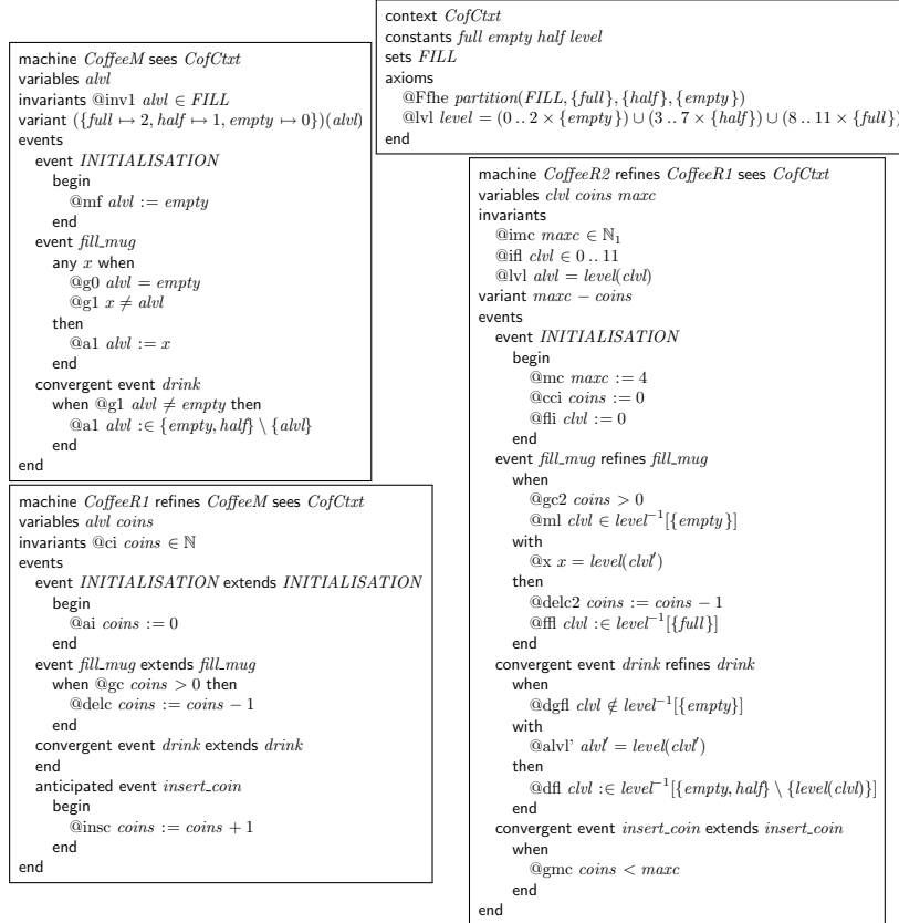
Fig. 1: Coffee dispenser model (using syntax of the Event-B text editor “Camille”) number of coins into the dispenser. A coin is consumed each time a mug is filled. In the second refined machine CoffeeR2 , the number of coins maximally accepted is limited and the amount of coffee contained in a mug is represented numerically by a the variable clvl (concrete level).
