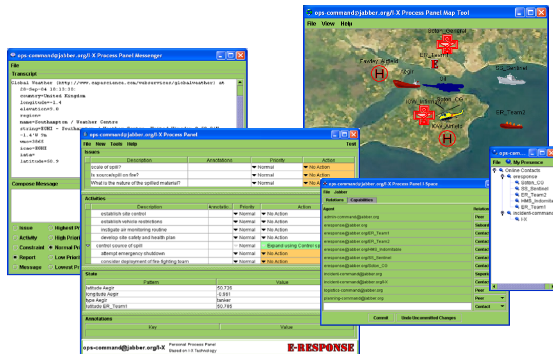
Figure 4. An I-X Process Panel, and its accompanying tools, shown here engaged in coordinating the response to a simulated environmental emergency [Image © AIAI]
