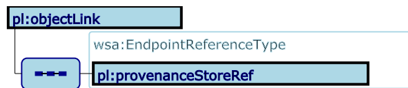
Figure 3: An WS-addressing endpoint reference pointing to the location of an object in a relation
