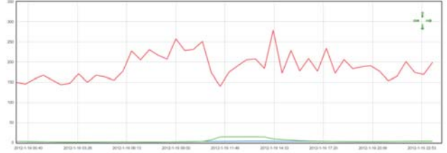
Figure 2: Load control in consumer sub-station (kW)
