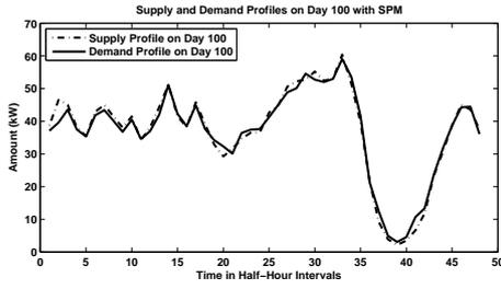
Figure 3: Supply Profile compared with Aggregate Demand Profile after the simulation has been run with SPM for 100 days
