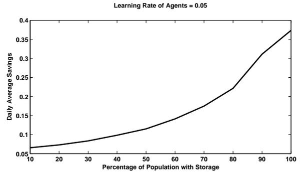
Figure 6: Average savings on electricity cost for consumers with storage and with electricity prices determined by SPM for different proportions of the population with storage.
