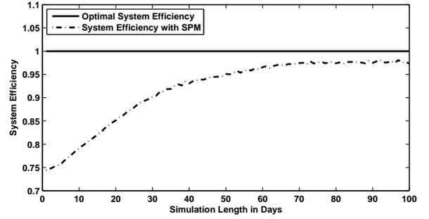
Figure 5: Storage efficiency of the system with SPM. At the start of simulation, the system is only 74.4% efficient
