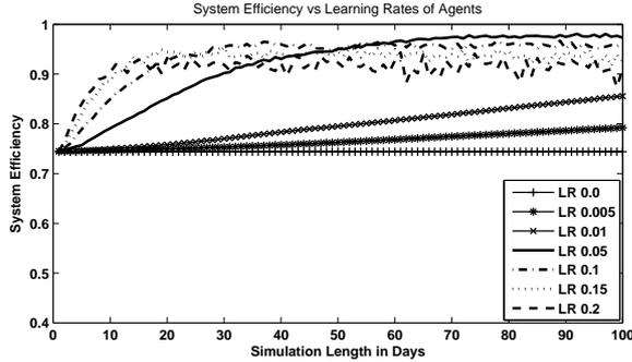
Figure 8: System efficiency for different learning rates of consumer agents and with electricity prices determined by SPM
