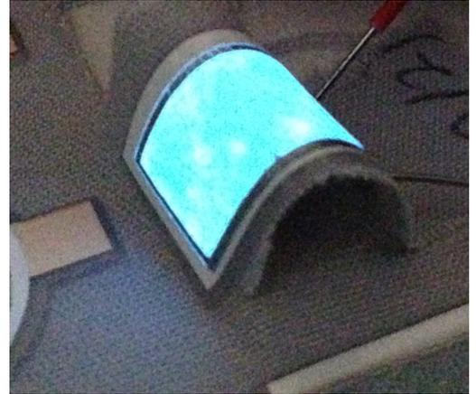
Figure 2: Screen-printed light blue EL lamp on fabric showing maintained fabric flexibility.
