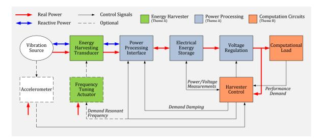
Vibration Source: Variable frequency and amplitude source of energy
