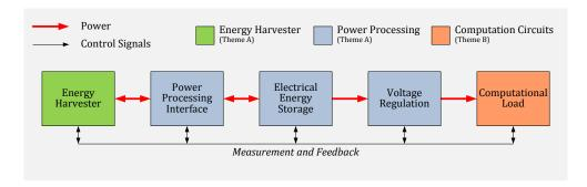
**Energy Harvester:** Power should be extracted from the source and converted to an electrical form. The ability may exist to allow the transducer to physically adapt (e.g. through frequency tuning) to maximise the harvested energy.
