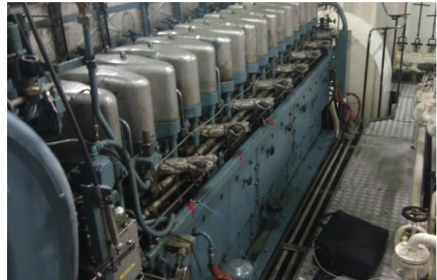
Fig. 2: Eight-cylinder diesel main engine on ferry
