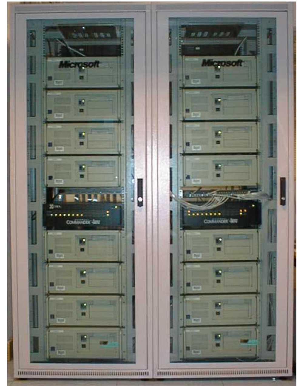
Figure 1. Microsoft Research (Cambridge) Cluster. Sixteen dual 300MHz PII's connected by Myrinet and switched fast Ethernet
