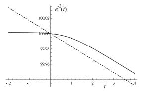
These plots show the effective electron charge as a function of  $\log(\mu/\mu_0)$  in the case of the MS-scheme, and for the momentum-subtraction scheme, with  $\ln(p/\mu_0)$ .
