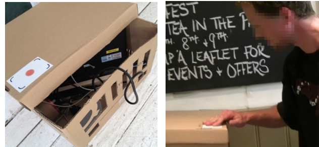
Figure 1. A game station (left) is a computer with an RFID reader and a target where players scan their RFID tags, and a player (right) swipes his ID on the box and awaits feedback.
