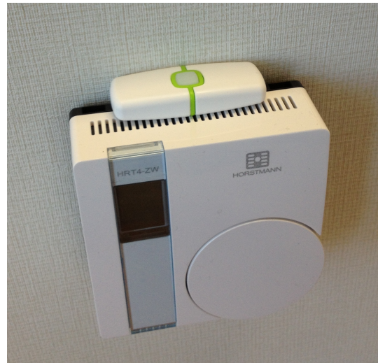
Figure 4: Deployed USB temperature logger.
