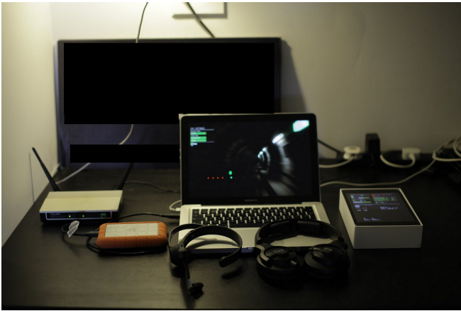
Figure 1. The components of the prototype system (left to right), WiFi router, Portable Harddrive with multimedia, Neurosky EEG Headband, Headphones, Laptop for viewing and iPad for controlling the experience.
