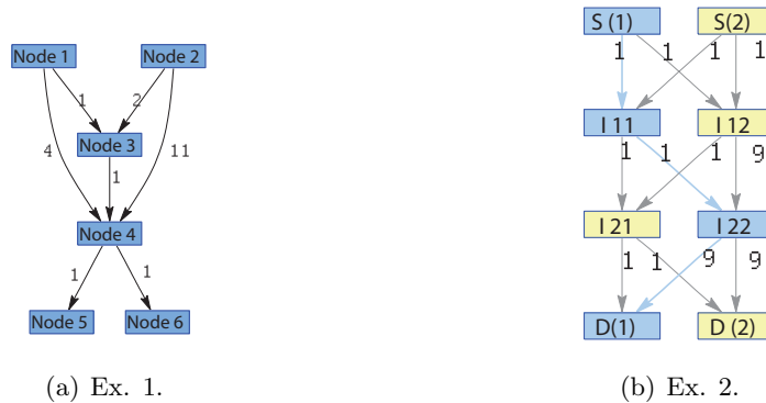
Figure 5.1.: Two examples. Numbers next to the edges denote the transition costs. Ex.2 : S(a)/D(a): start/destination of agent a. Coordinated plans depicted in blue (Agent 1) and cream (Agent 2) which happens to be socially optimal.
