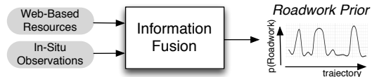
Fig. 1. This paper is concerned with the data fusion of web-based resources (websites citing the expected locations of roadworks) and in-situ observations (detections of roadwork indicators in Fig 2) to estimate a roadwork prior.
