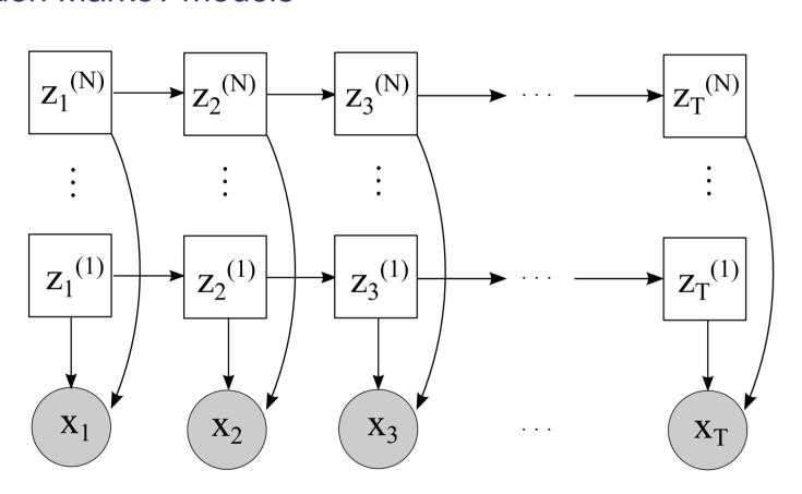
z<sub>t</sub><sup>(n) –</sup> hidden state of appliance n in time slice t x<sub>t</sub> – observed sum of emissions in time slice t
