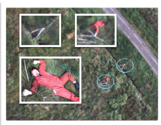
Possible targets viewed at altitude trigger closer inspection to discriminate between targets and clutter.
